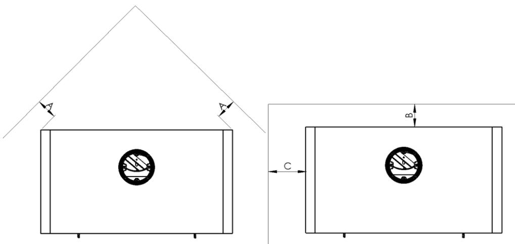
**If a non-combustible board is laid under the stove, it must protrude at least 50 cm off in front of the stove and 30 cm off at each side of the fireplace opening.**
